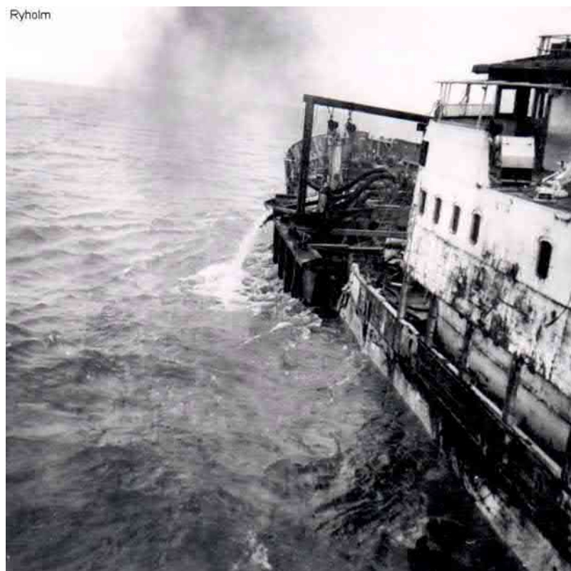
8. The new steel patch in place, pumping begins to refloat Ryholm .
